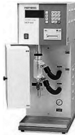
Figure 9: Automatic Fiber Optical Freezing Point Apparatus for test method ASTM D7154 (Source: www.astm.org )
