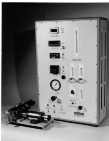
Figure 12: Semi-Automatic Ball-on-Cylinder Lubricity Evaluator for test method ASTM D-5001 (Source: www.astm.org )
